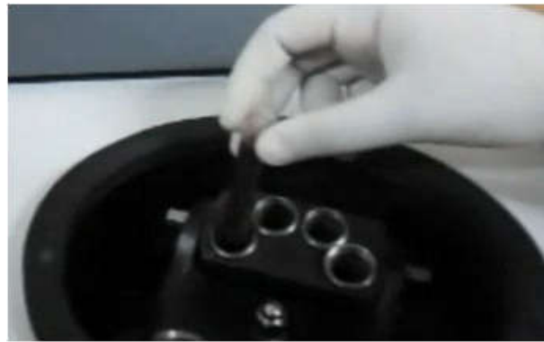
Fig. 9b: Centrifugation tube containing blood is being placed in centrifugation machine
